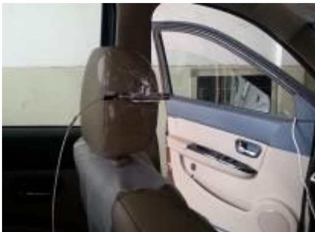
FIGURE 2 The install location of microphone in driver’s right ear
